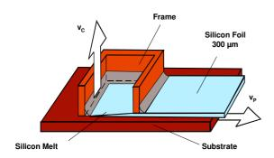
**Figure 1**: Principle of the RGS wafer production technique.
