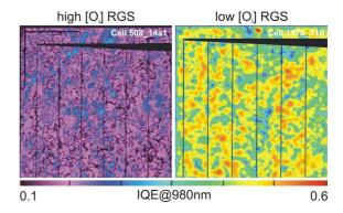
**Figure 8:** LBIC maps of two RGS solar cells (photolithography based cell process) from RGS wafers with different interstitial oxygen concentrations. The right mapping is a high resolution detail (upper left corner) of the cell shown in Figure 6, left.
