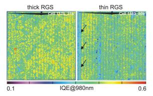
**Figure 6:** LBIC mappings of the same RGS solar cells as presented in Figure 4 and Figure 5 (photolithography process). The line marked with arrows in the right measurement indicates the range of Al screen printing.
