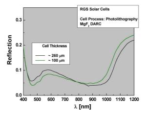
**Figure 5:** Reflection curves of two of the RGS solar cells as presented in Figure 4 (photolithography based cell process including a SiN / MgF<sub>2</sub> DARC).
