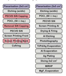
**Figure 2**: Solar cell processes applied to RGS. Left: Industrial-type firing through SiN screen printing process. Right: Photolithography based high efficiency process including screen printed Al BSF, hydrogenation and double layer antireflective coating (DARC).
